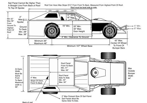
78" Maximum Body Width At Bottom Of Panels Near The Ground. You Are Not Allowed To "Flare" Bottom Edges Of Panels And Exceed Maximum Measurement Shown.
