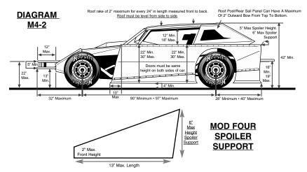
down to a maximum of 2" tall at the front of the spoiler support. May be 6" tall for a maximum of 8" forward from the top of the spoiler, then taper down to 2" at front of spoiler support. This will be measured with a template. Maximum of three (3) spoiler supports. If you use sail panels for supports, you can have one additional spoiler support. No other spoilers, wings or ground effects are allowed anywhere outside or inside the car except for on the nosepiece side panels.
