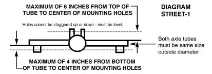
Must not be adjustable. No weight jacks allowed. No added traction devices allowed. Leaf springs must be stock or replacement; must use original mounts; no adjustable shackles allowed. Lowering blocks allowed on leaf spring cars only. Lowering blocks must be steel. Refer to diagram Street-1 for rearend mounting locations.
